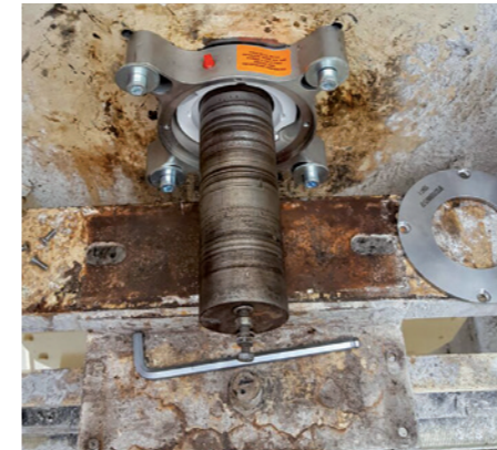
End cover and O-ring mounted on the machine wall
